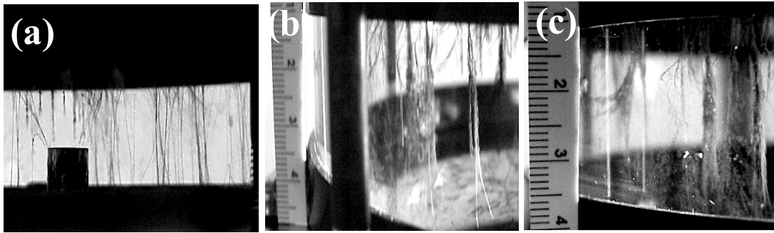
Figure 26. Photographs of FeAl filaments in the chamber ( E = 60 \text{ V/cm} ) after 30, 60 and 120 min in a, b and c, respectively.
